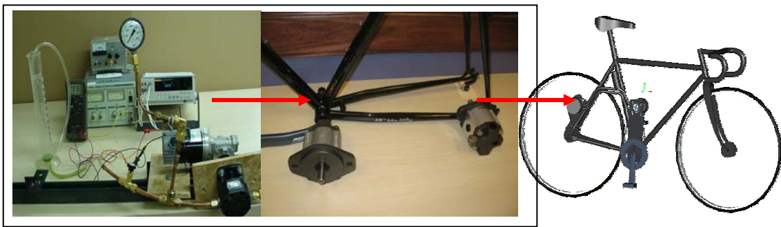
Figure 2. Transition of the Design Abstraction: From Simulation of the Hydraulic Bike System to Construction
