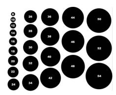
The measuring tool features a series of circles starting with a diameter of 8 mm with each subsequent circle increased in size by two millimeters to a maximum of 54 mm. The advantages of using the circles to measure the rocks are that it is cheap, quick and easy, and allows a sufficient degree of accuracy in measuring each rock at its longest point. This is also a good opportunity to remind students of the "True-Score Theory" (all measurements
