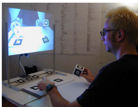
Figure 4. System set-up with a typical situation of use: charging the Gripper with an element from the booklet (left). The platform (right) holds an unsaturated atom, with which a binding with the charged atom may be triggered (Fjeld & Voegtle, 2002).
