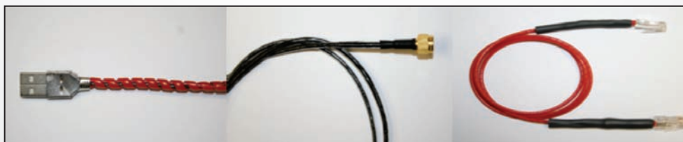
Fully Functional CNT cables from left: USB, Coaxial, and Cat 5 Internet cables.
