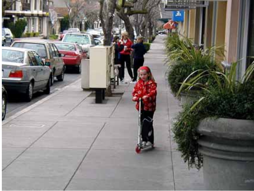
Figure 9-4. Photo. Parked cars can also serve as a buffer between the sidewalk and the street.
