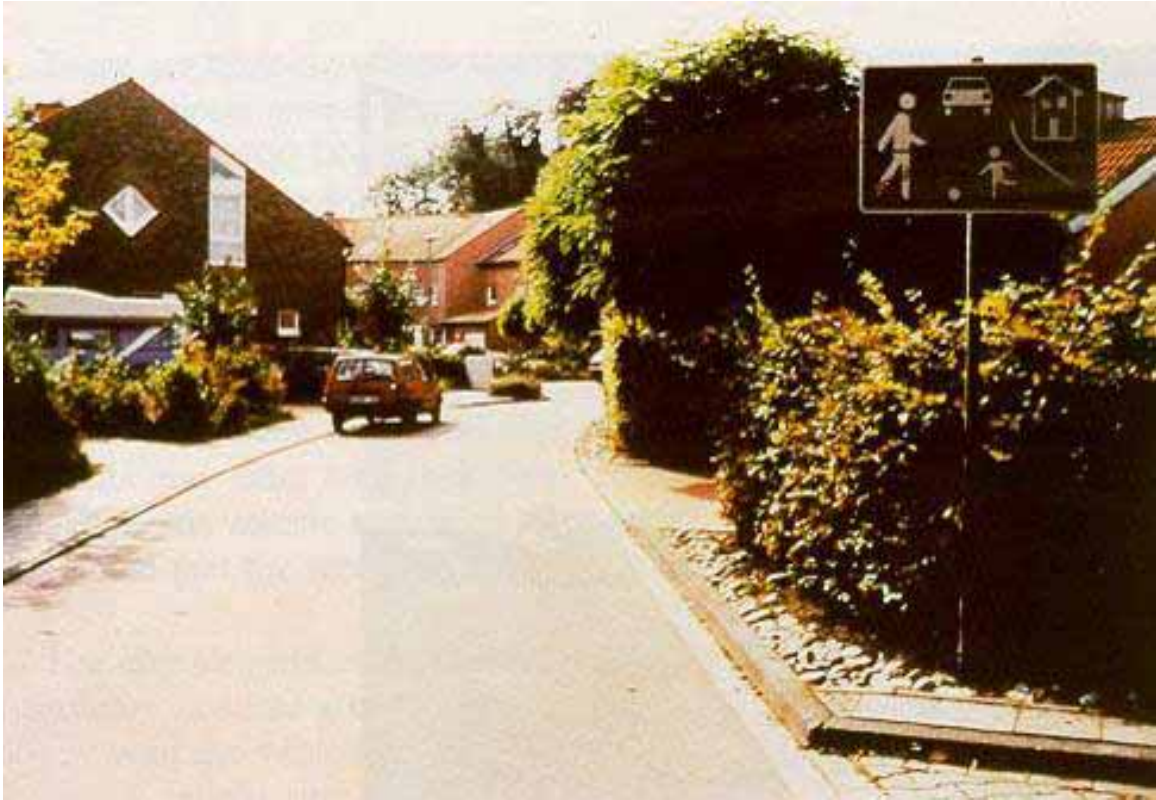
Figure 20-20. Photo. The distinctions between sidewalks and roadways are blurred in woonerfs.
