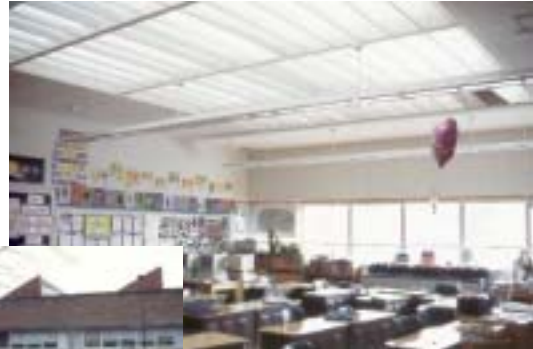
Central sawtooth monitor provides even illumination across desks in this classroom. NREL/PIX 11406
