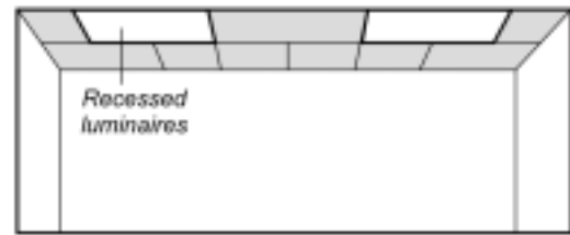
Recessed luminaires are direct general light source.
