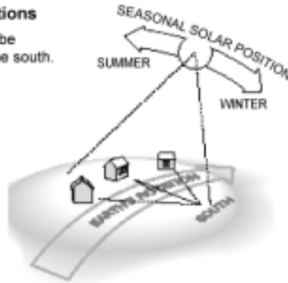
Figure 38 – Solar Positioning Considerations
