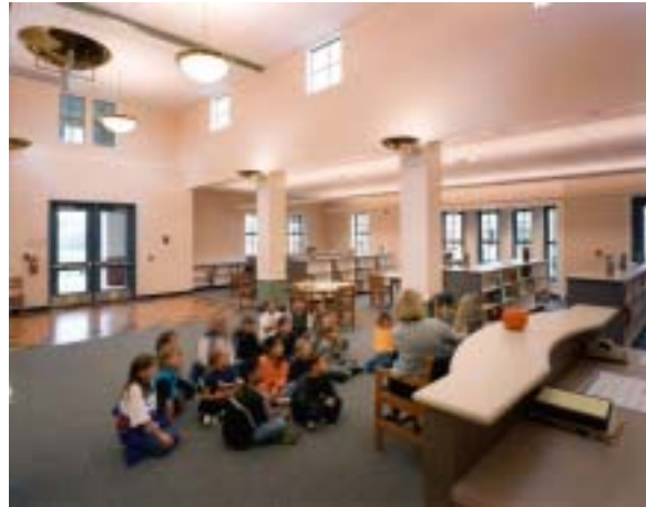
This library uses a combination of daylighting for ambient light and task lighting above desks and card files. NREL/PIX 11439
