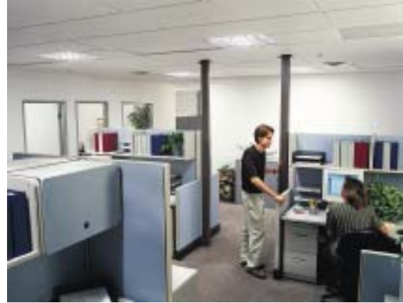
Tubular skylights in interior administrative office provide high lighting levels even when electric lights are off. Skylight diffuser panel fits into a standard suspended ceiling system.
