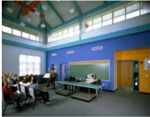
Clerestory windows provide a more uniform distribution of daylight across the space. NREL/PIX 11404
