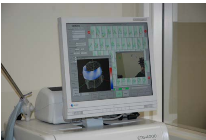
Figure 2. Computer portion of the Optical Topography system
