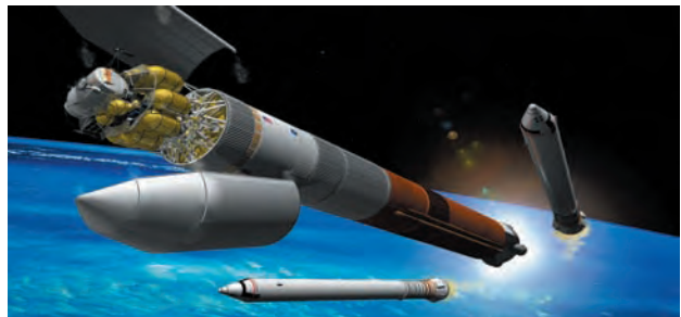
Ares V lifts the Earth departure stage and Altair lunar lander to orbit.
