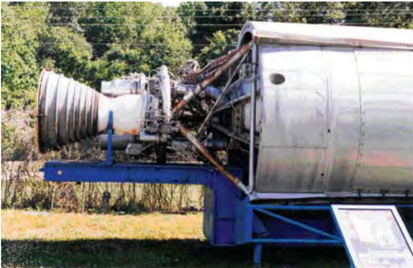
Actual The Engine and Thrust Structure of a Titan Rocket
