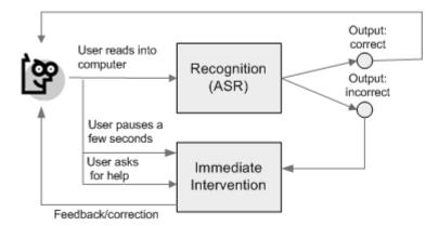
Figure 1 A general scheme of immediate intervention in speech recognition application to facilitate learning to read correctly for dyslexic children
