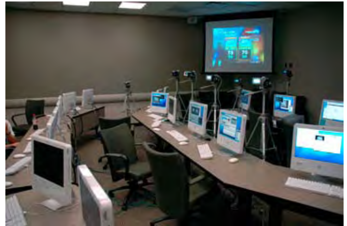
This is the setting of the testing site. All server machines are in the back row. All broadcasting machines are in the front two rows, each connecting to an external video camera looking at an HD video signal on a big screen.
