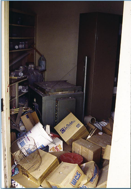
Figure 4-28 Damage to ceramic kiln, including fractured gas line, Northridge, CA, 1994
