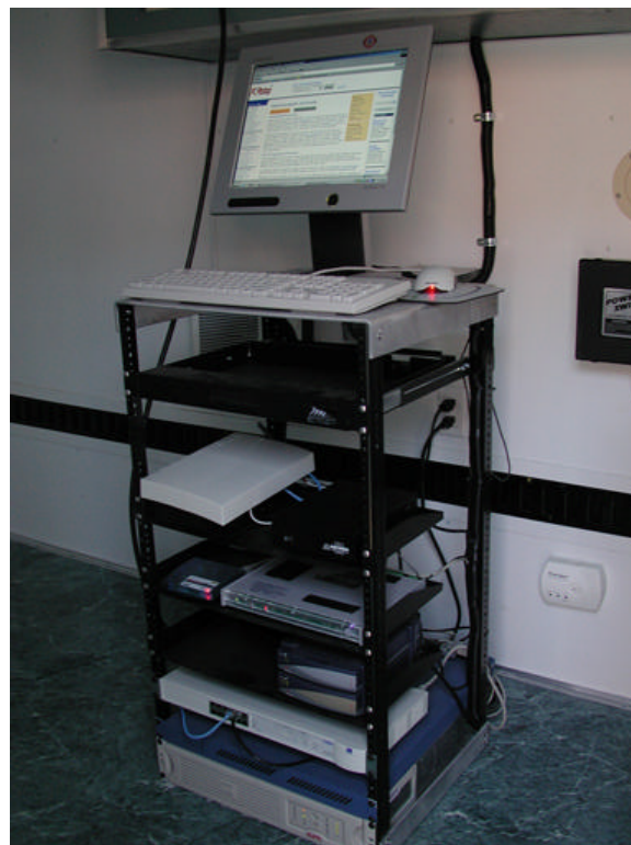
Figure 5: The satellite control unit and computer network switch
