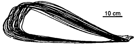
Fig. 2 Step trajectories measured at the ankle with (black line) and without (grey line) ARTHuR attached. Twenty steps are shown for each case.
