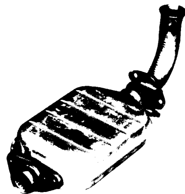
This lightweight catalytic converter is typical of those found in many newer-model automobiles.
