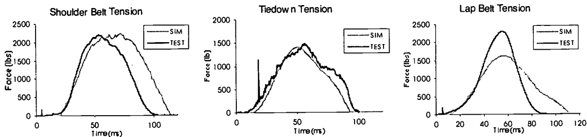
Figure 2: Computer simulation output (SIM) and sled test data (TEST) harness and tiedown data comparison
