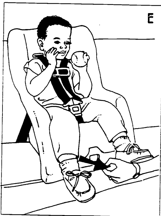
The harness on this convertible seat is tightened by pulling on the strap between the child's feet.
