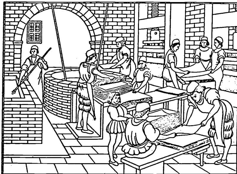
The vatroom of a paper-mill at Fabriano in the middle of the 15th century. All the processes are shown in detail; the sheet being made on the mould; a sheet being couched on to the felt; boys parting the sheets from the felts; men parting the sheets from each other; and the great presses.
