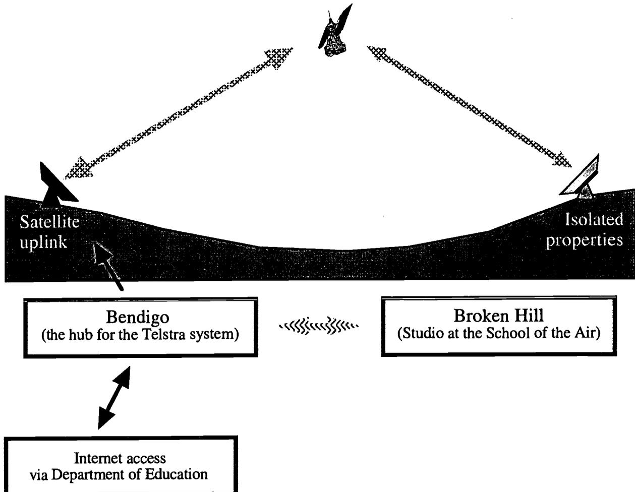
The system under which the *Satellite Trial* at Broken Hill took place is illustrated by Figure 2. The studio was set up at Broken Hill and broadcast lessons to the students via the *Telstra* facility at Bendigo in northern Victoria. The signal from Bendigo was then transmitted via the satellite to each of the participating properties as well as the window sites.
