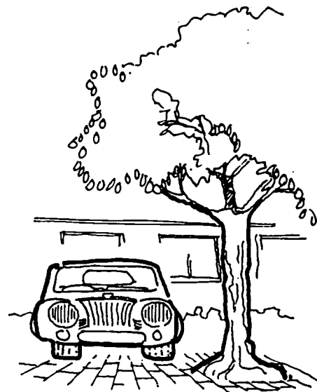
UNIT PAVING UNDER TREES REDUCES IMPACT OF TREE ROOTS ON PAVING AND ASSIST GROWTH
