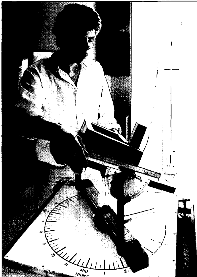
Figure 30: Use of model in conjunction with a heliodon.
