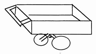
This type of cart has a payload of 2-3 cubic meters, is frequently made of wood, can have bicycle wheels or other small vehicle wheels, and the axle is usually metal, as is the handle. Some sort of metal framework around the base of the cart holds it together and makes it more sturdy.
