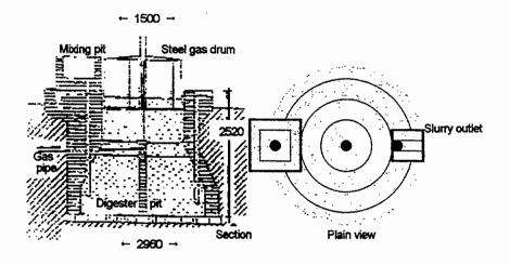
Taper design of steel drum biogas plant
