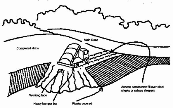
Strip width 6 metres; only one vehicle at a time on working face; capacity 30-40 tonnes/day.
