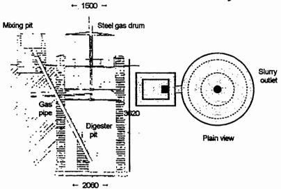
Straight design of steel drum biogas plant
