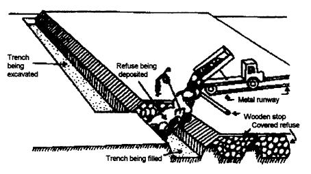
The trench method of controlled tipping. The heaps of refuse are lievelled and formed to a 45° slope using a long-handled rake, and covered by at least 150 mm of soil excavated from the next trench. The width of the trenches should not be less than their depth. Source: After Flintoff (1984).
