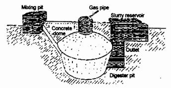
Fixed dome design of biogas plant
