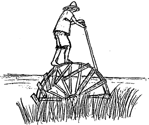
Figure 2: Man-powered water wheel for irrigation
