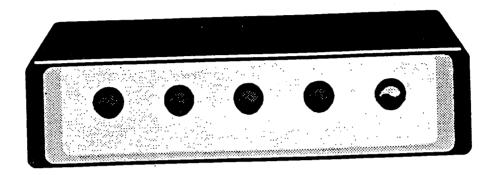
The modem is an internal or external device that connects the computer and a phone line. It converts computer (digital) signals to phone (audio) signals and vice versa so that information can be sent and received over the phone lines.
