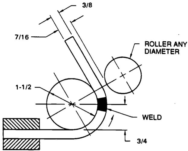
**Figure 9 - Alternative Wrap Around Bend Test Fixture**
