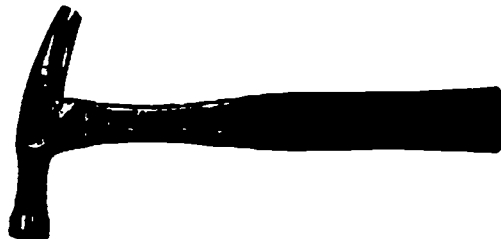
Figure 1-56 Can be used to mount electrical boxes and drive nails. Can also be used to determine height of receptacle box since most hammers are 12" in length from head to end of handle, or can be so marked. (Klein Tools, Inc.)
