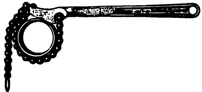
Figure 1-68 Used to tighten and loosen larger pipes and conduit. (Courtesy of The Ridge Tool Company)
