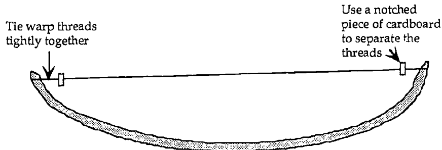
Figure 17a: Bow loom from the side. A string is wrapped tightly around the two ends of the stick, making the stick bend. Keep wrapping until at least five warp threads travel from one end to the other. Notching the stick will keep the warp threads from slipping. The warp threads are tied together tightly near the bow ends. A piece of cardboard with one notch per warp is inserted, with each warp thread firmly pushed into the corresponding notch; the notches on this cardboard should be slightly farther apart than the width of a bead.
