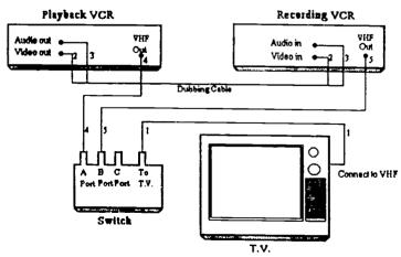
\* NOTE \* Double check to make sure all plugs fit tightly and correctly.
