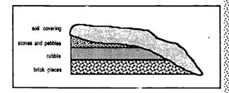
The height of each slope may be 50 cm and the length of the ridge 100-150 cm, with a gentle slope on one face (see fig).
