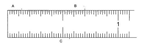
e.g. Read the following measurements on the enlarged decimal-inch rule shown above:
