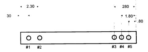
For example: In the drawing above, holes #1 and 2 must be measured only from the left edge. Hole #3, 4 and 5 must be measured from the right edge.
