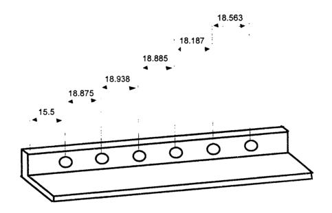
The blueprint is shown below. The tolerance for all measurements is  $\pm .125$  inches. Find the upper and lower limit for each dimension on the blueprint below. Compare these limits with the measurements given above. Which holes are drilled incorrectly?
