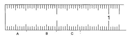
e.g. Read the following measurements, to the nearer graduation, on the enlarged decimal-inch rule shown:
