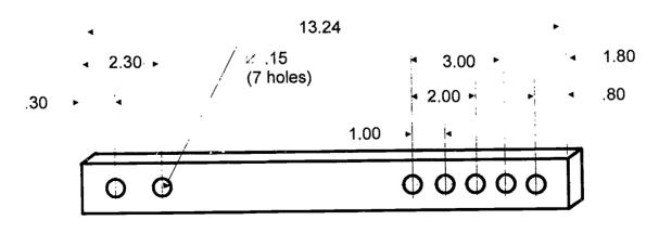
24. What is the spacing of the holes from center to center? (The holes are evenly spaced.)
