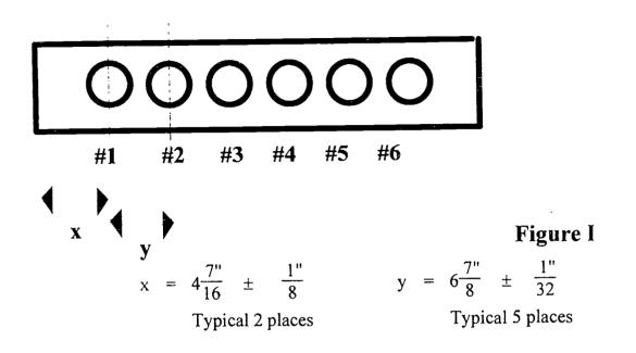
A machinist drills the holes and checks them for proper location. The actual locations of the drilled holes are shown in Figure II. Which holes are drilled out of tolerance?
