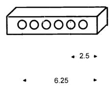
25. Find the missing dimensions. The hole is placed in the center of the plate. The radius of the hole is .56 inches.
