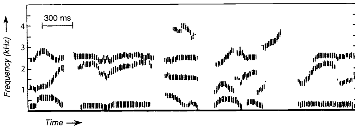
Figure 1. Spectrographic representation of the tone replica of the sentence, "My t.v. has a twelve inch screen." Amplitude variation is represented in the height of each hatch mark placed at the tone frequency.
