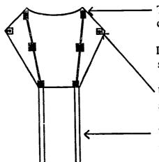
Tape dowl rods from top point to bottom corner, securing at top, middle and bottom.
