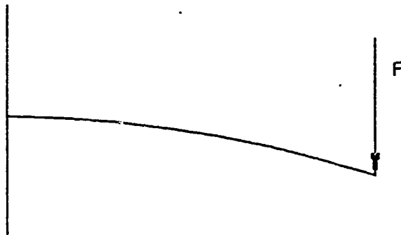
Figure 4 Cantilever Beam Loading
