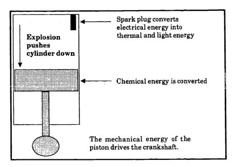
Energy is put into the system. The chemical energy of gasoline drives the piston. This is called input energy. The electrical energy that drives the spark plug is another form of input energy. Chemical energy is transformed into mechanical energy which moves the car. The mechanical energy used to moved the car is output energy. The car converts or transforms the chemical energy into mechanical energy.
