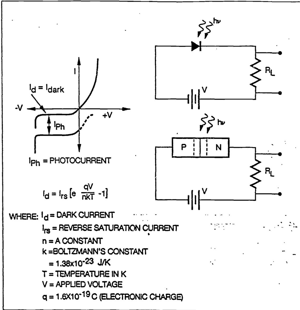
FIGURE 51 Dark current in semiconductor photodiode
