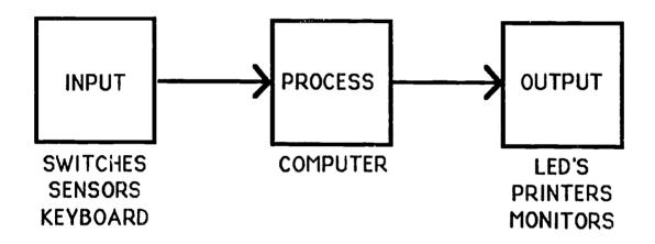
Computer interfacing contains three major systems. Input is information being put into the computer. The computer looks or reads locations connected to external devices. Typical devices used for input include sensors, switches, and keyboards. Once the computer processes the information, it must then output it to the world outside the computer. Typical output devices include LED's, buzzers, printers, and video monitors.
