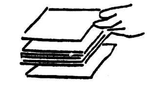
STEP 2 - Fasten the pages together by stapling or sewing by hand, or using a machine on the longest stitch. Machine sewing offers more durability.
