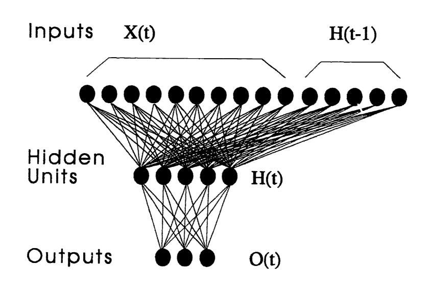
Figure 2: A recurrent network structure
