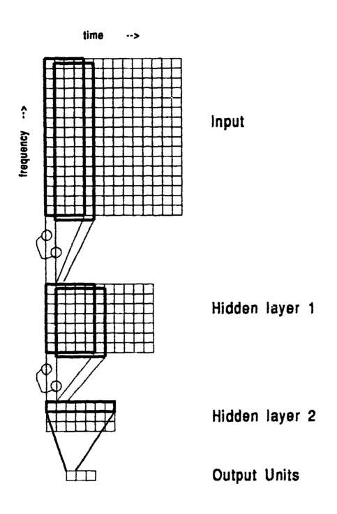
Figure 3: The Time Delay Neural Network structure
