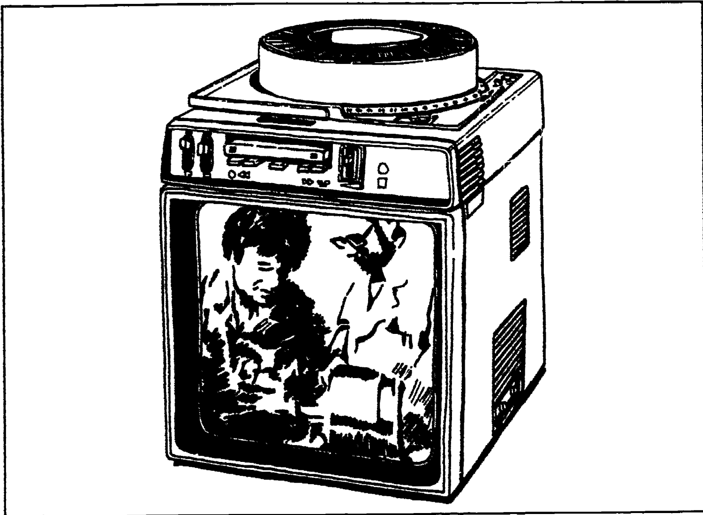
Figure 7.7 Self-contained unit for slide-tape presentation
