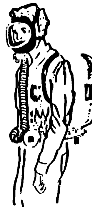
Typical open circuit SCBA.
