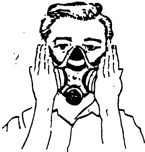
NEGATIVE PRESSURE TEST
