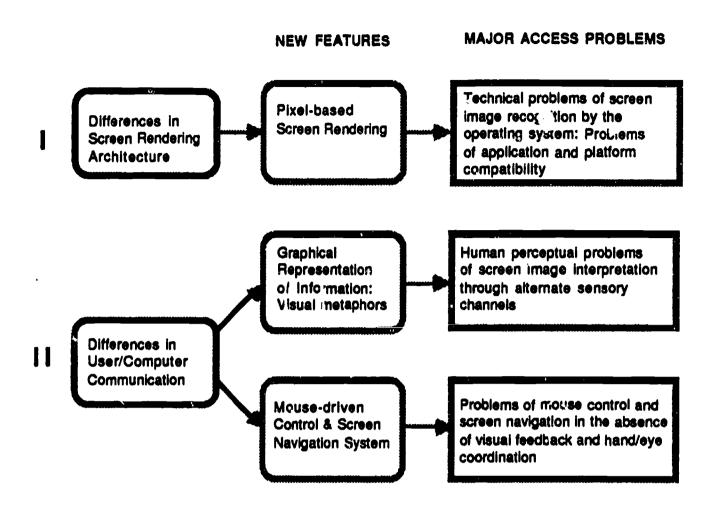
Figure 1. Major Differences Between the GUI and Traditional User Interfaces With General Categories of Features and Access Problems for Blind Users
