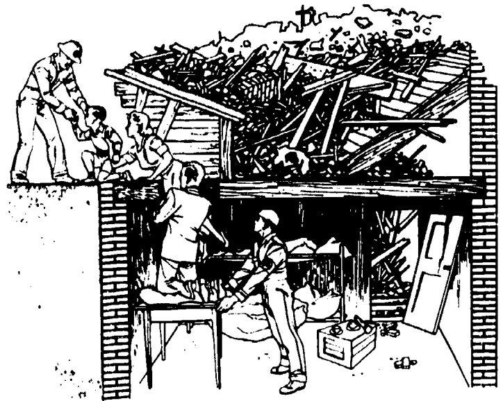
Figure 16. Tunneling to Gain Entrance
