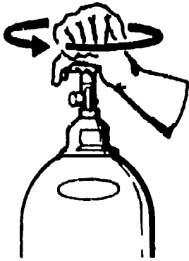
Figure 44. Cracking a Cylinder Valve
