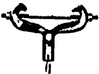
malleable beam clamp with extension piece fig. 229; without, fig. 218 safe load: 610 to 1365 lb.
