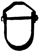
adj. clevis fig. 260 1/2 to 30 in. pipe light weight clevis fig. 65, 3/4 to 4 in. pipe adj. clevis for C.I. pipe fig. 590, 4 to 24 in. pipe
