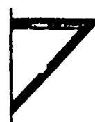
welded steel brackets medium fig. 195 max load: 1500 lb.; heavy fig. 199 max load: 3000 lb.
