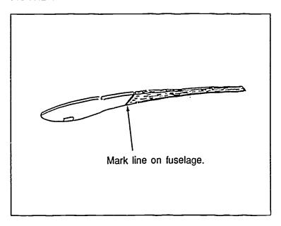
d. Spread glue evenly over back surface of right and left paper fuselage pieces (see Figure 7-a) and then quickly glue paper fuselage pieces to balsa fuselage as they were test-fit in step b above (see Figure 7-b)
