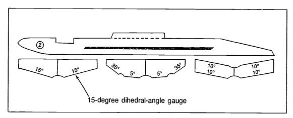
b. Rough-cut and then trim exterior lines of angle-gauge piece
