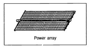
(NOTE: A series of eight power arrays will provide electric power aboard the space station during its early years. Each array will consist of two blanket assemblies, each covered with 14,592 solar cells.)
