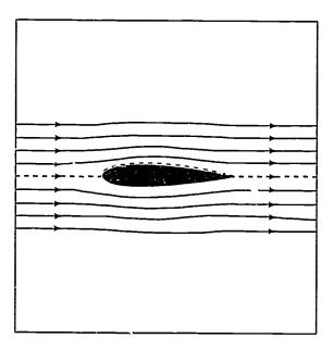
With a wing of the typical shape shown in Figure 1, the upper surface of the wing is thicker than the lower surface. Since the wing's upper surface is thicker, the speed of the air flowing over the upper surface is greater than the speed of the air flowing over the lower surface. The difference in the speeds of the two airflows causes a greater pressure to be exerted on the lower part of the wing than on the upper. This difference in pressure causes the upward force needed to create lift.
