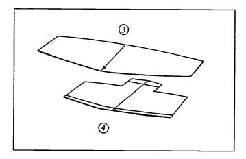
e. Set assembled wing aside and allow glue to dry for at least five or six hours
