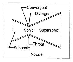
During operation, gas velocity in the convergent part of the nozzle is subsonic. Gas velocity increases to sonic speeds at the throat and to supersonic speeds in the divergent portion.
