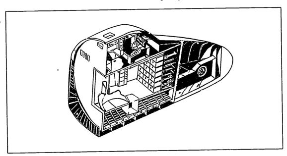
The orbiter's two-story crew cabin contains a flight deck on the top level and living quarters underneath. This cutaway view shows the left side of both stories. Redrawn with permission of NASA, John F. Kennedy Space Center.
