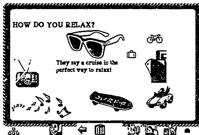
Figure 11.13: The Relax card. Each picture is cover by a transparent button which puts text relevant to the picture into the central field.
