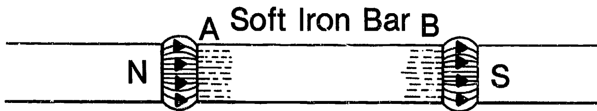
Magnetizing an Iron Bar by Induction
