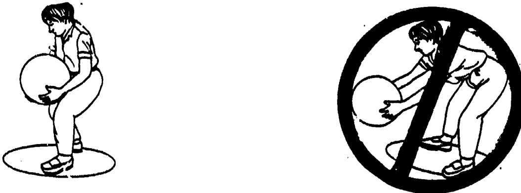
Figure 3.4 This figure shows on the left a person working within her safe work space. On the right the person by moving out of her safe work space is risking injury to her back.
