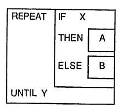
In any execution (application) of this FLOWform, condition X is tested first. If X is true, operation A is carried out; otherwise B is executed. Next, condition Y is tested. If true, the process terminates. If Y is false, the above process (the body of the "loop") is repeated until Y becomes true.
