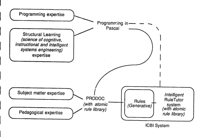
Figure 1. --- Schematic depicting IMS approach to intelligent ICBI (tutor) development and high level structure of ICBI system.
