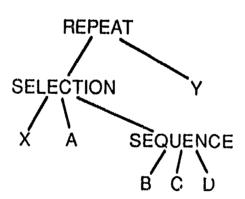
In the above picture, X and Y are conditions and the operations A, B, C and D are atomic rules. The equivalent ordered set representation of this procedure is as follows:
