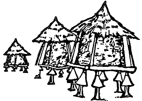
Fig. 50 Traditional nkhokwe improved with rat guards and muddying, Malawi
